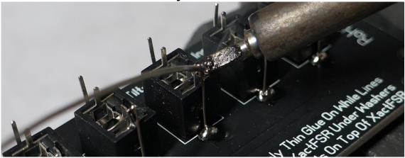
8. reinforce the pad solder joints
