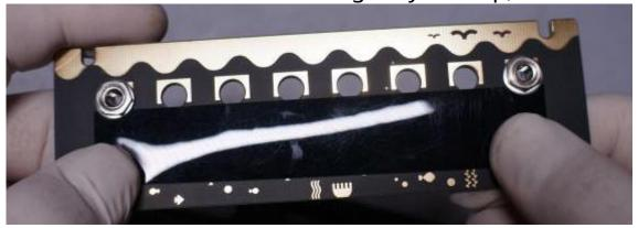
3. tighten the nuts and install all jacks, make sure they align with silkscreen
