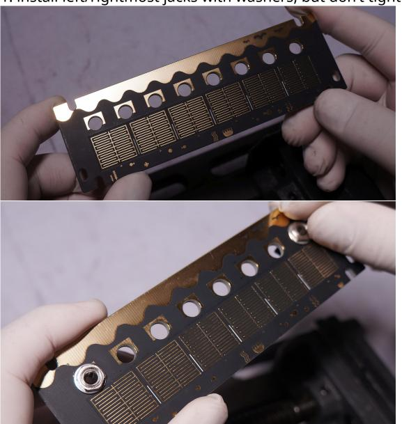
2. slide the XactFSR sheet with glossy side up, underneath the washers
