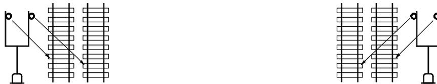
Where a track intervenes between a signal and the track governed, a dummy mast, marked by a blue light or reflector, will be placed to the field side of the signal.
