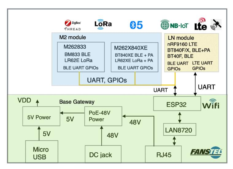
Open Source IoT Gateway supporting multiple radios, multiple networks
