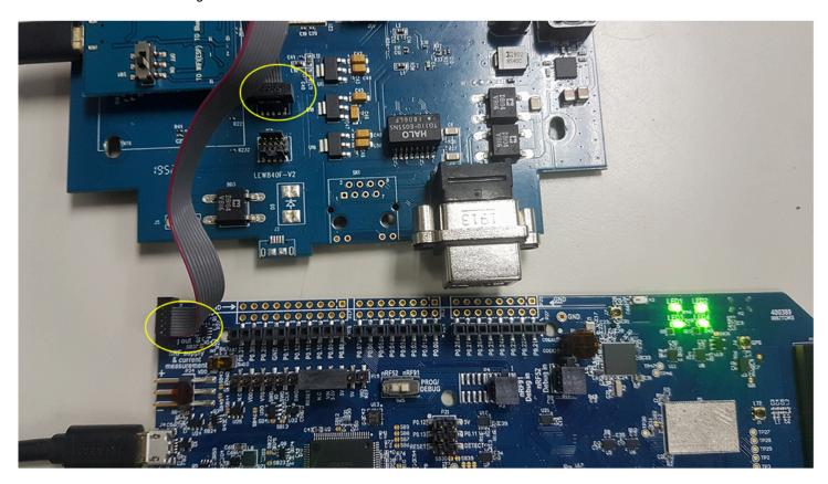
Open nRF connect /programmer and load the softdevice and application. Erase and write.
