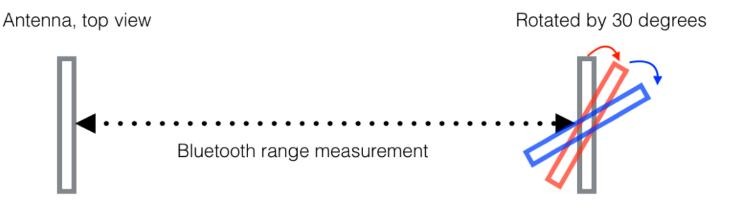
Bluetooth range is specified as the average of 12 measurements with the least significant digit truncated.
