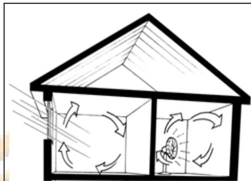
*Natural ventilation rates are highest in winter because cold outside temperatures cause high stack pressures in the house. The higher the pressures, the more infiltration and exfiltration. It is true that some houses see higher natural ventilation rates in summer if they keep their windows open wide. This changes the house air-leakage area. Natural ventilation rates in summer with windows closed can be very low.*
