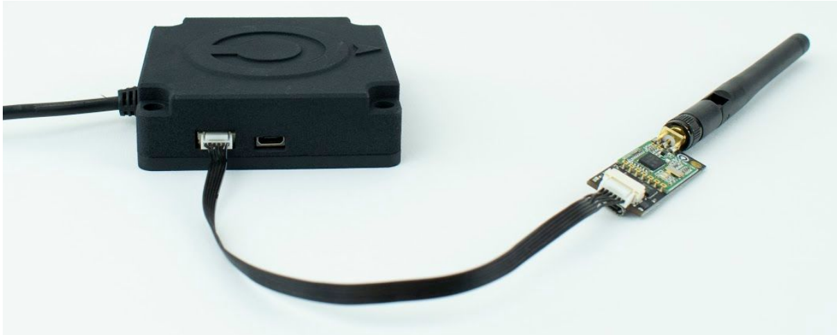
Figure 3. Sirius F9P Rover connected to a 433MHz telemetry kit using UART2
