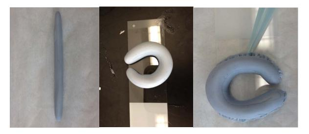
21. Carefully place the sample in between the Blu-Tack pieces and add about 20  $\mu L$  of FocusClear to the sample.
