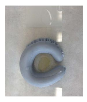
22. With the lipped side facing up, firmly press a Willco dish down onto the adhesive until it just comes into contact with the sample. Using a pipette, add more FocusClear to the gaps between adhesive until the imaging chamber is filled.
