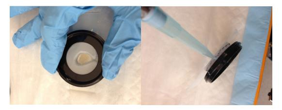
23. KWIK-SIL is an adhesive that cures rapidly. Carefully add it to the gaps between the Blu-Tack to build a wall and seal in the sample. Take care not to introduce any bubbles, and make sure the chamber is completely filled with FocusClear.
