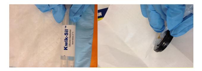
24. Cover this construction with aluminum foil and store it away safely to cure. After about 20 minutes, the sample is ready for imaging.
