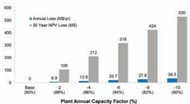
Figure 2. Annual capacity factor is often the vital factor in a project's success. The net present value is based on a 30-year term and 5% discount rate.
