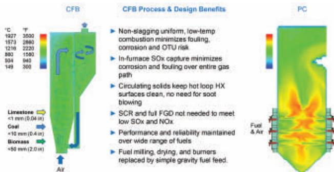
Figure 1. The low temperature operation of the CFB reduces NO<sub>x</sub> emissions and limestone injection into the bed removes SO<sub>2</sub>.
