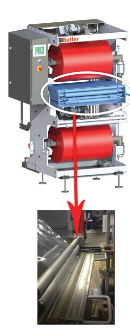
Splice is created by melting and sealing two rolls of material together without tape
