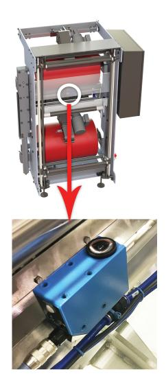
Splice is actuated when a pre-applied contrasting colored tape on the web is detected by the end-of-roll sensor
