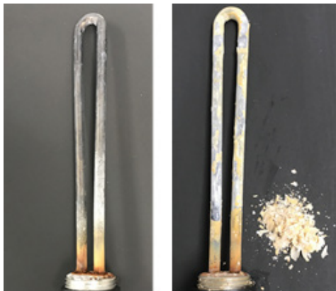
Figure 4. Scale prevention results of TAC vs. Technology B
