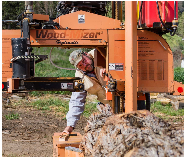
Kendall turning Juniper logs into dimensional lumber. Bottom photo credit: Marcus Kauffman.
