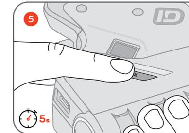
5. Hold the Delete (“x”) button for 5 seconds to delete the selected profile.
