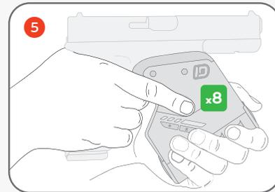
5. To capture a fingerprint profile, press your finger onto the scanner 8 times.
