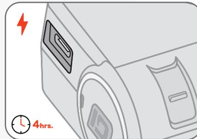
Prior to using IDENTILOCK, charge the unit until the status indicator light turns green (up to 4 hours).
