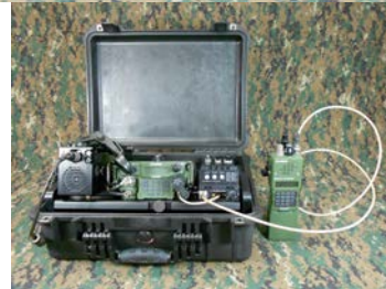
TCR-MPR-01 with secondary radio connected to auxiliary RF port.
