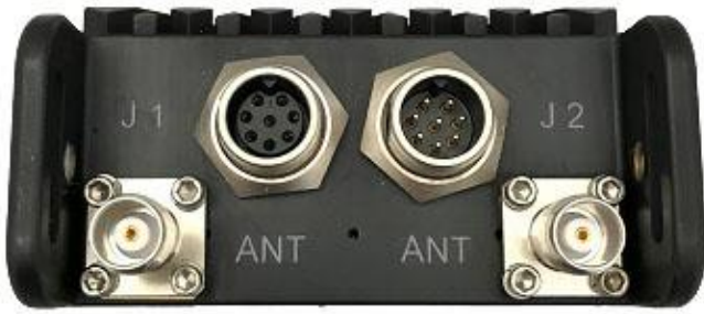
RADIO TOP VIEW CONNECTORS AND TnC PORTS
