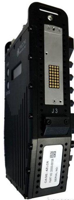
RADIO SIDE VIEW 32 PIN SIDE CONNECTOR
