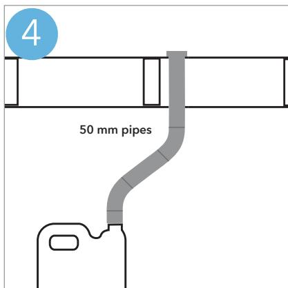
**Install a urine outlet with 50 mm piping to a urine container of your choice. Push down the pipe sleeve to the floor and fix with silicon.**
