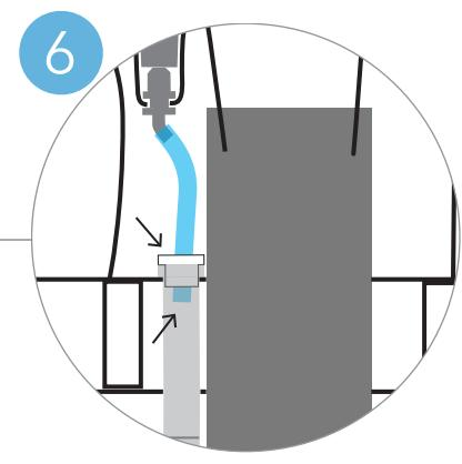
**The white adapter on the urine hose should be pushed down tight.
