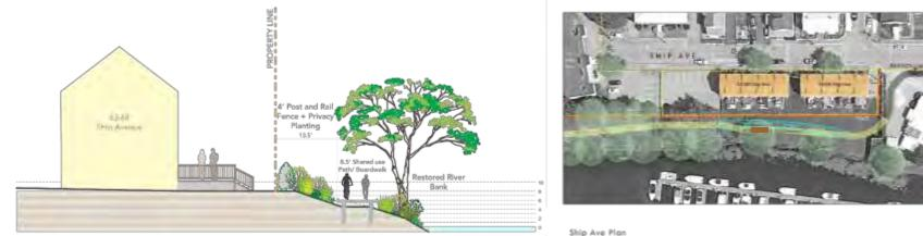
Shared Use Path Section at 62-68 – NEW ALIGNMENT PATH SHIFTED 5 FT AND BOARDWALK AT TREE TO MINIMIZE TREE IMPACT)
