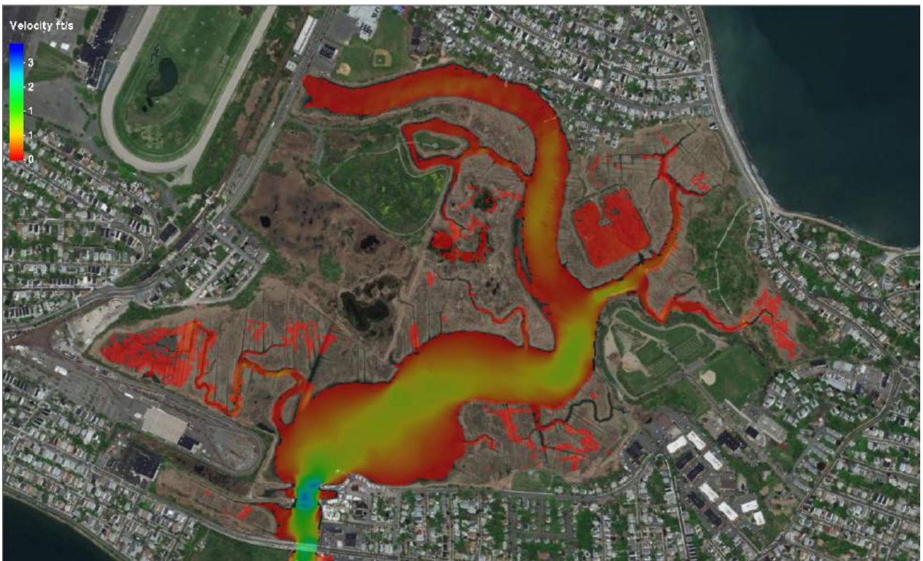
A2. Existing Velocities, typical Neap Tide Ebb. Velocities are reported in feet/second, with high velocities indicated in blue.
