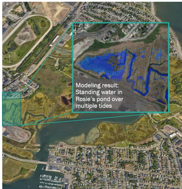
Figure 34. Example EFDC model results depicting tidal perching in Rosie’s Pond during a spring low tide.
