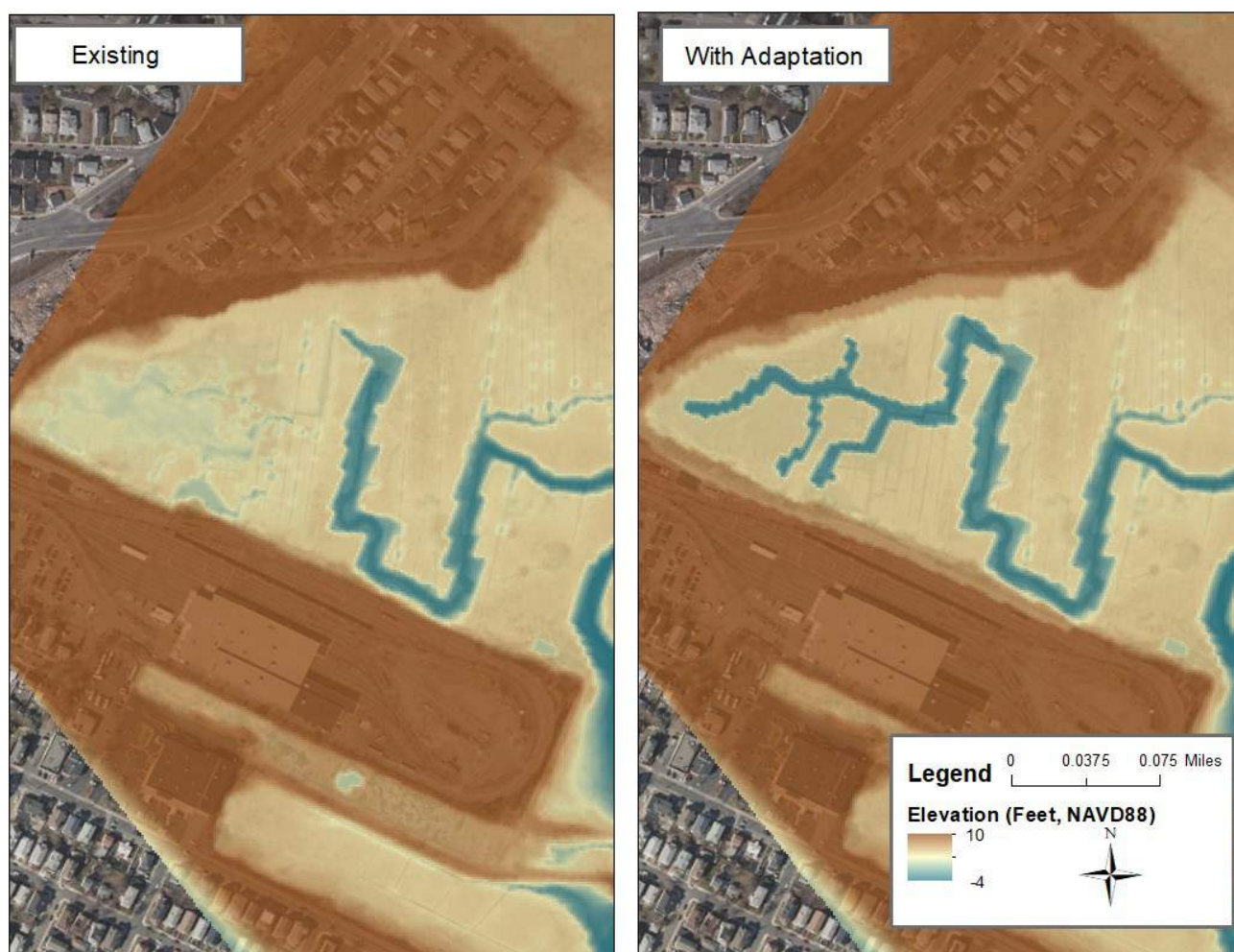
Figure 23. The left panel presents the existing conditions, while the right panel presents the restoration scenario for the Rosie's Pond sub-region of Belle Isle Marsh. Higher regions are presented in orange, brown and yellow, whereas low regions are presented in shades of blue. All elevations are in feet, NAVD88.
