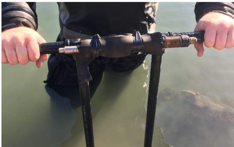
Figure 9. An aqua troll A200 mounted on a pipe anchor prior to deployment.
