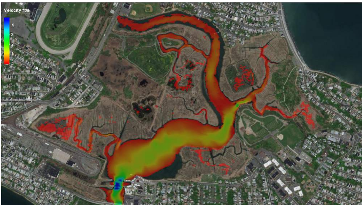
Figure 8. Existing Velocities, typical Spring Tide Ebb. Velocities are reported in feet/second, with high velocities indicated in blue.
