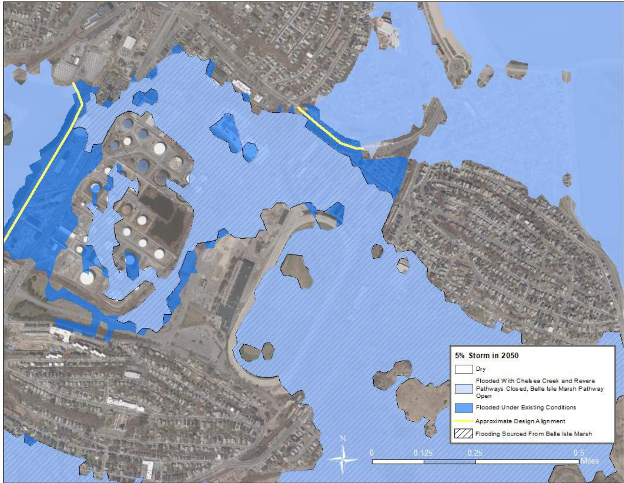
Figure 8. Extents of flooding for the 5% Storm in 2050. The light blue indicates areas that are flooded in both existing and when the Revere and Chelsea Creek Flood pathways are closed (flooding contribution from Belle Isle Marsh), whereas the dark blue regions indicate areas of avoided flooding due to the Revere and Chelsea Creek flood pathways. The yellow line indicates flood pathways that are blocked in the model simulation.
