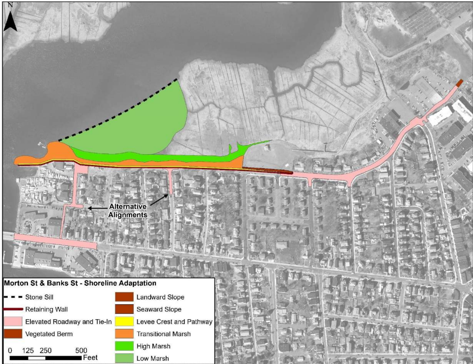
Figure 11. Morton St – Living Levee and Elevated Roadway.
