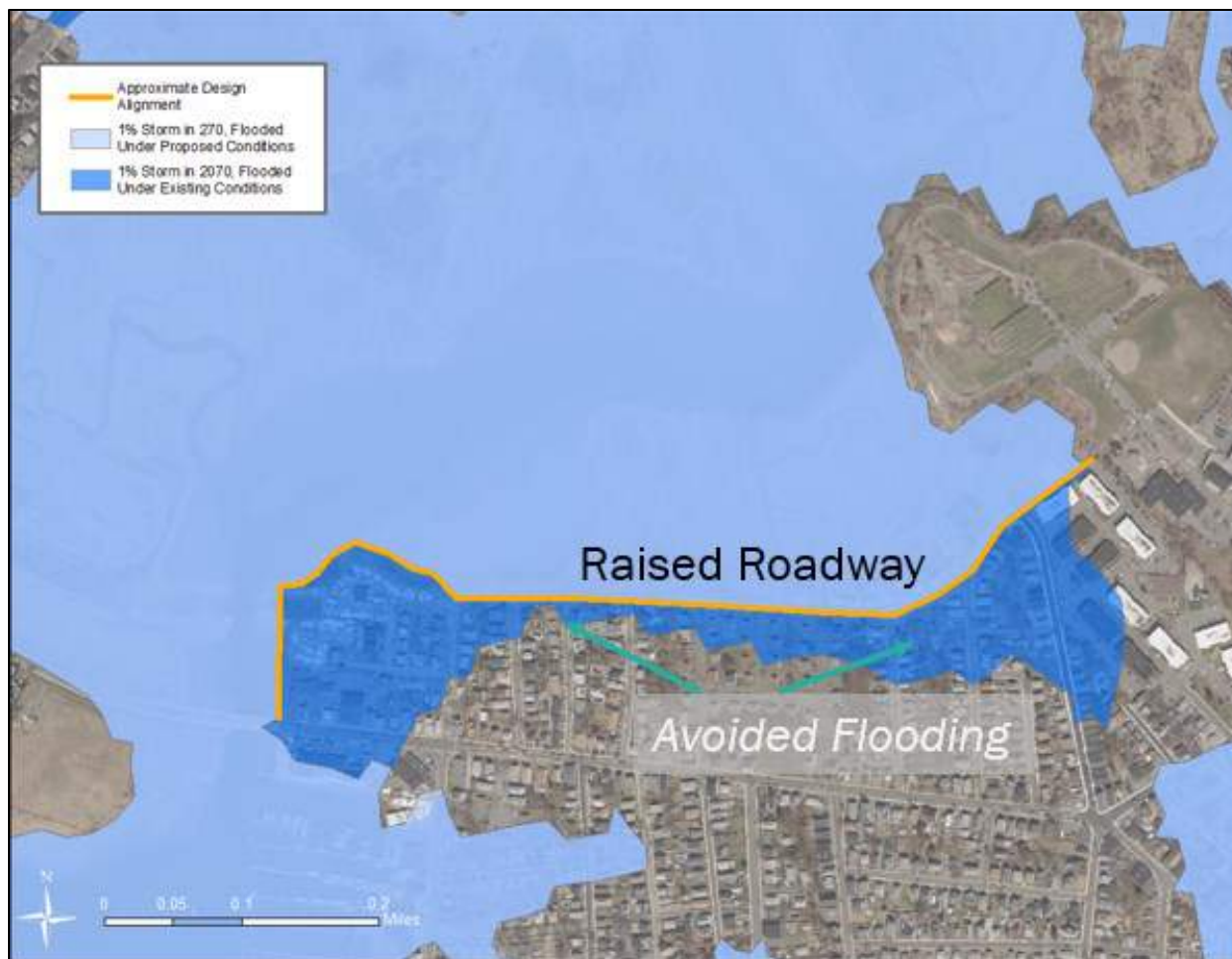
Figure 11. A 2070 1% event results for existing and proposed conditions, with a living levee constructed along the edge of Belle Isle Marsh, tying into an elevated Morton Street (elevated crest elevation of 14.1 ft NAVD88). The light blue indicates areas that are flooded in both existing and proposed conditions, whereas the dark blue regions indicate areas of avoided flooding due to the design alternative. The orange line indicates the approximate location of the alignment crest.
