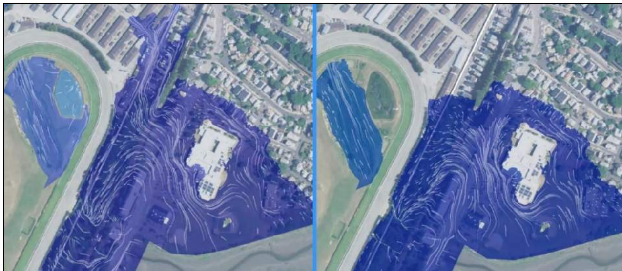
Figure 9. Flowpath and current velocities under a “No Build” (left) and “Full Build” (right) condition which includes the HYM development, pump station upgrades, installation of a berm at Washburn Ave, construction of flood storage within the proposed development. Scenario depicted represents 1.5 ft of sea level rise, a 100-yr rainfall event, and a 100-yr tide event (VHB, 2018). Impacts to Bennington St and adjacent public assets such as the MBTA Blue Line and Revere Public Schools are not significantly mitigated by the “Full Build” condition.
