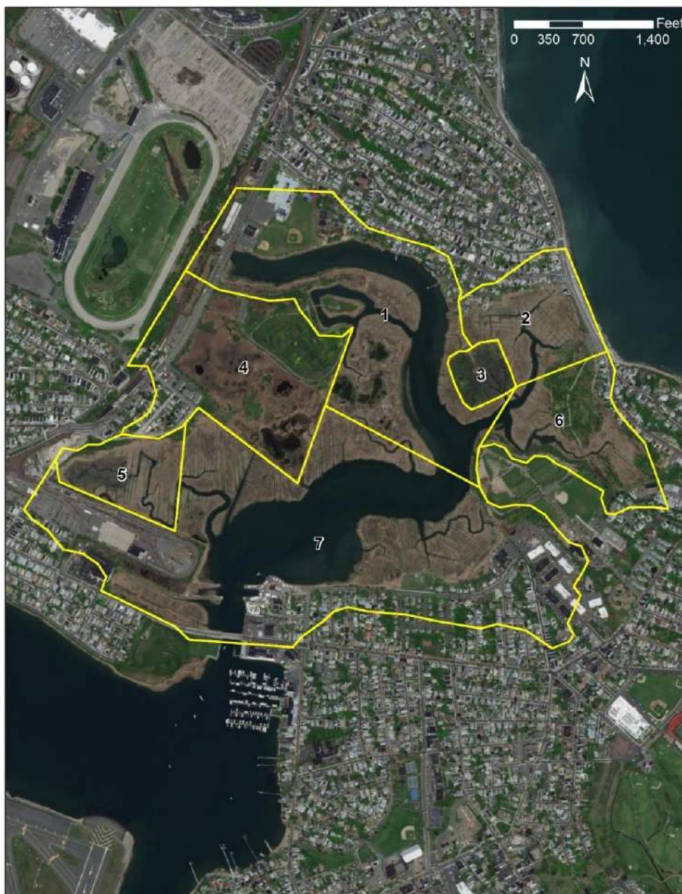
Figure 4. Sub-sites delineated for SLAMM based on the hydraulic conditions present within Belle Isle Marsh.
