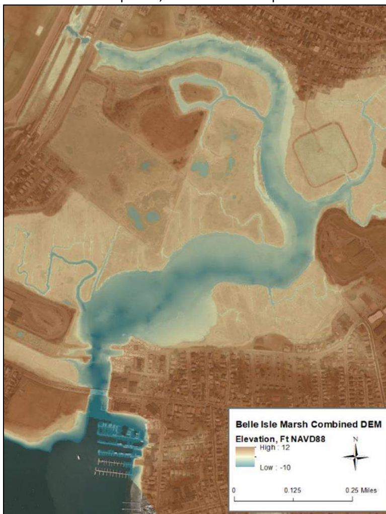
Figure 2. Combined Topobathymetric DEM used for hydrodynamic modeling, overlain on 2018 Orthoimagery for Massachusetts. All elevations are reported in ft, NAVD88.
