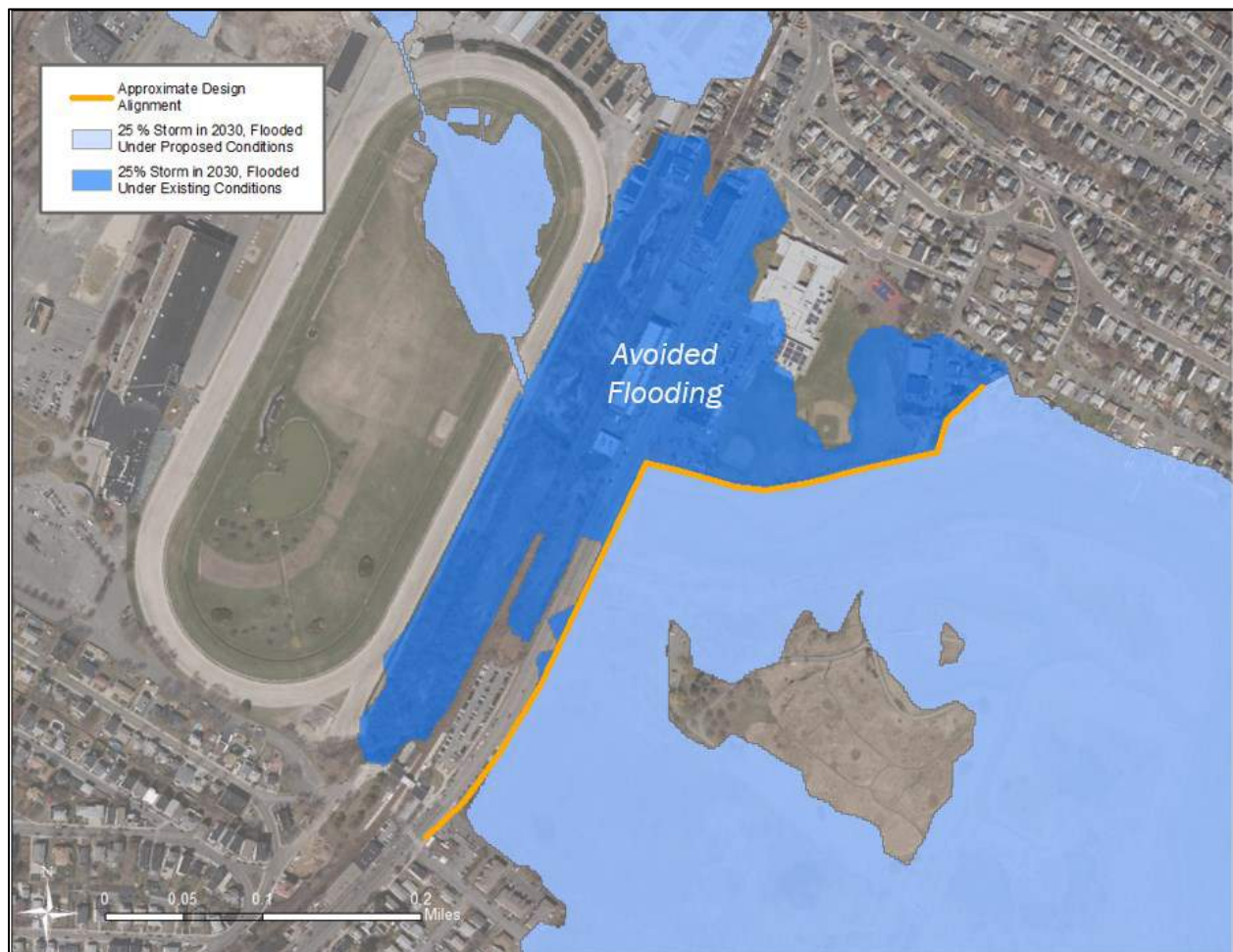
Figure 6. A 25% storm under the 2030 time horizon (equivalent to the 1% Storm in Present Day) results for existing and proposed conditions, with an extended elevated Bennington Street, and flood protection berm on the Belle Isle Marsh-facing side of Frederick's Park (crest elevation 14.1 feet). The light blue indicates areas that are flooded in both existing and proposed conditions, whereas the dark blue regions indicate areas of avoided flooding due to the design alternative. The orange line indicates the approximate location of the alignment crest.
