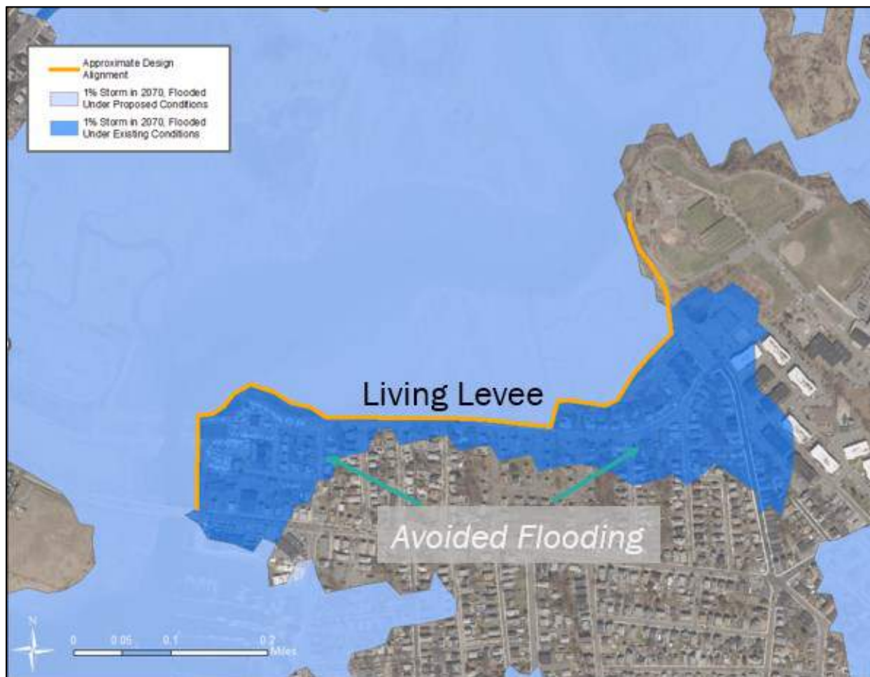
Figure 10. A 2070 1% event results for existing and proposed conditions, with a living levee constructed along the edge of Belle Isle Marsh in the Morton Street region (elevated crest elevation of 14.1 ft NAVD88). The light blue indicates areas that are flooded in both existing and proposed conditions, whereas the dark blue regions indicate areas of avoided flooding due to the design alternative. The orange line indicates the approximate location of the alignment crest.
