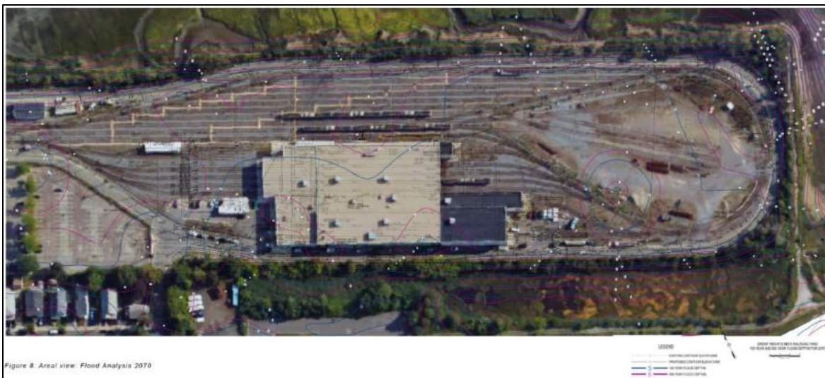
Figure 7. Sea level rise and storm flood projections in 2070 for the MBTA Orient Heights maintenance yard. The 100-year flood depth (blue contour) and 500-year flood depth (purple contour) depict flooding across the majority of the railyard. Under the 2070 predicted storm event, the facility could not continue to function (AECOM, 2018).
