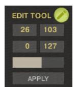
slider controls the curve of the line being edited. The bottom slider switches between the line curve types and direction.
