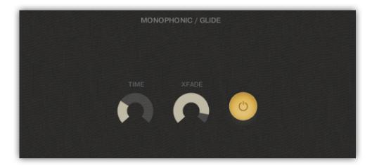
The time dial lets you choose the duration of the glide, while the xfade dial lets you choose the duration of the fade between the current and the new note that was triggered, achieving a smoother transition between the two samples.
