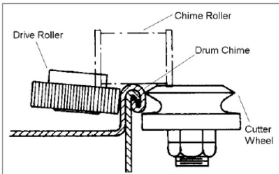
These models were designed specifically for the food industry and are USDA approved. The outside chime cut protects the drum contents from contamination and allows access to 100% of the drum contents. Lid stays in place until ready to lift off with the Wizard cover lifter. Lid can be reused as a cover.
