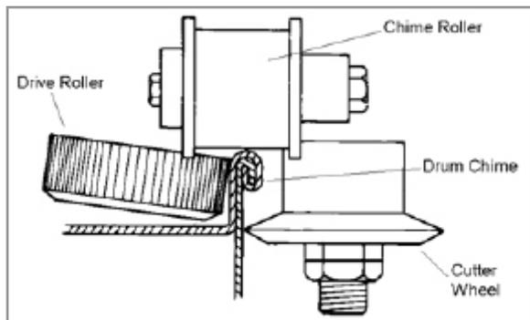
Wizard model specifically designed for scrapping drums. These deheaders cut on the outside of the drum shell so smooth, dent-free chimes are not required. Remove the entire drum top and/or bottom for drum flattening. Flattened drums take up less space and prevent potential liability from future drum use
