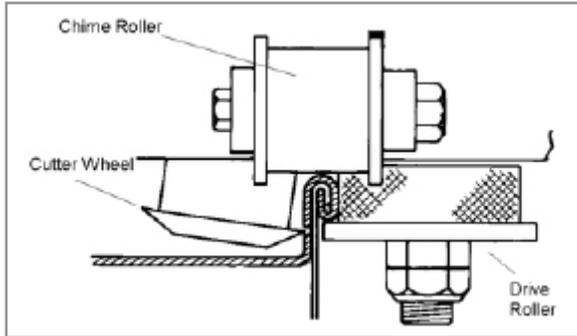
The most versatile and popular Wizard models. cut on the inside of the rolled edge and leave a smooth, burr-free "hand safe" edge. Ideal for deheading both storage, shipping and utility containers. Also can easily remove both drum tops and bottoms for drum disposal.
