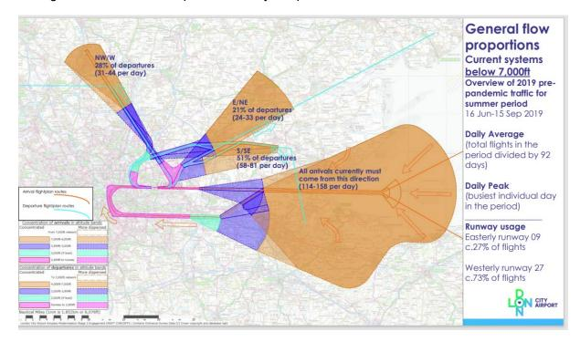
The observed aircraft for this study vary in altitude above Mean Sea Level (MSL) from around 2400ft/740m in Mottingham in the east to 2000ft/610m at Horniman museum in the west. However London City aircraft have been recorded on the airport's tracking system as low as 1600ft/488m above MSL along this flight path.
