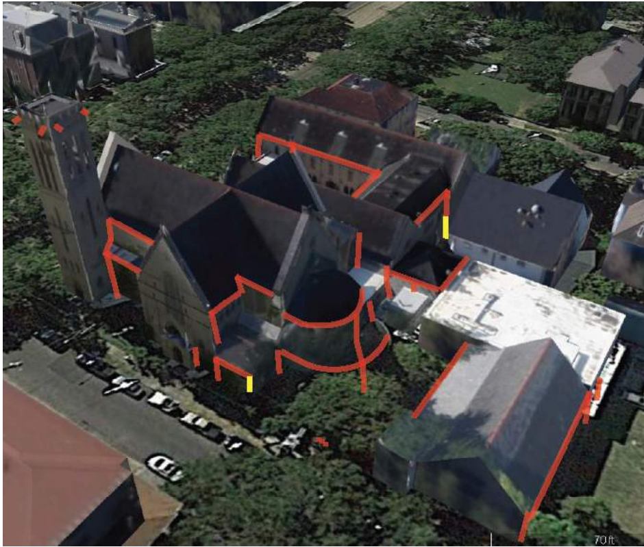
Figure # 6.3: On this aerial view of the church, gutters and downspouts are mapped in red, missing gutters and downspouts in yellow. Photo by Google Earth, Edits by Nathan Lott, 2015
