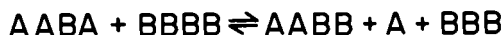
Figure 7.5 An exchange reaction involving cleavage of two old bonds and formation of one new one.
