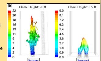
Flame length was reduced by over 50% for the proposed case and There was a significant reduction in radiant tube metal temperature.
