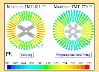
Existing heater operation was limiting on draft with positive pressure of 0.1 inches WC at arch. Also, it was required to increase the heater duty by 40%.
