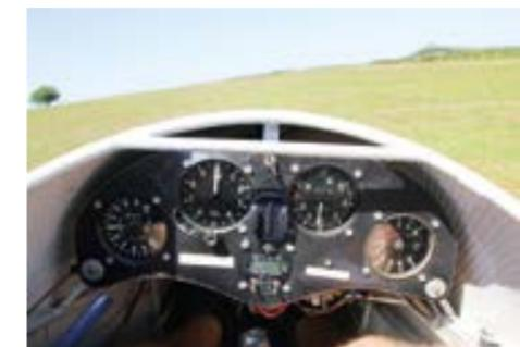
CLOCKWISE FROM TOP The Dartmoor landscape stretches out beyond the glider just after take off; The basic cockpit of a glider displays everything you need to know when in the air: speed, height, vertical speed and speed across the ground; The graceful, almost silent landing of a glider towards the end of the day
