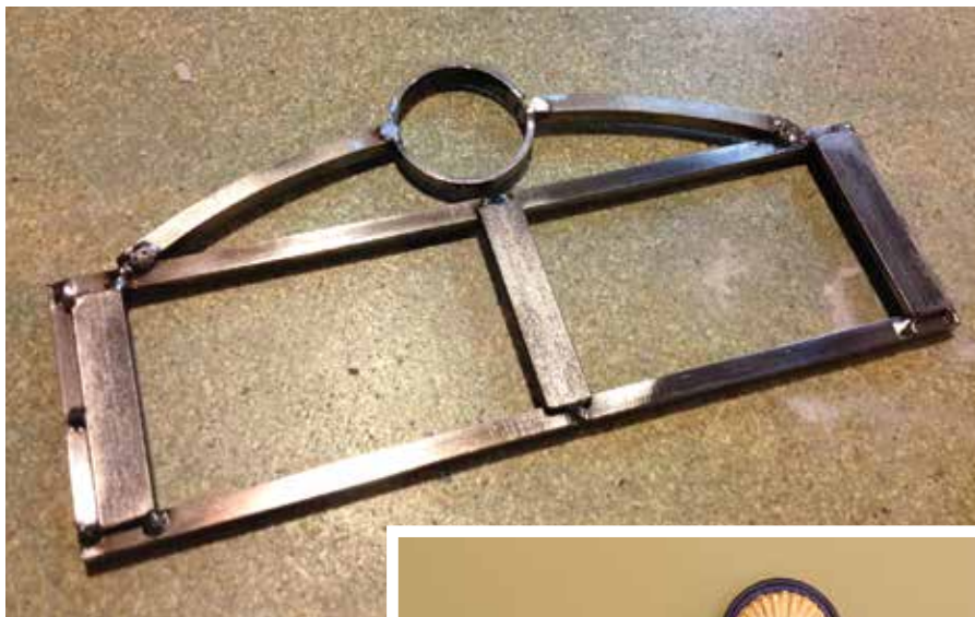
A steel frame for the Parish Office ADA sign.
