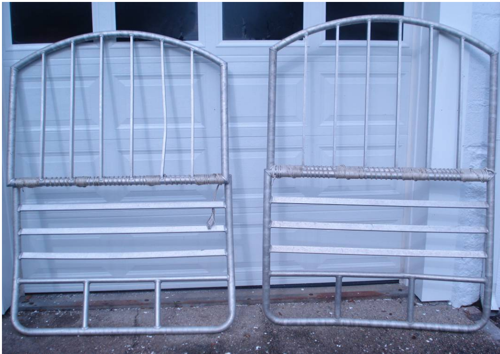
Figure 5b. Photograph of the northeast modified TED showing damage from being used.
