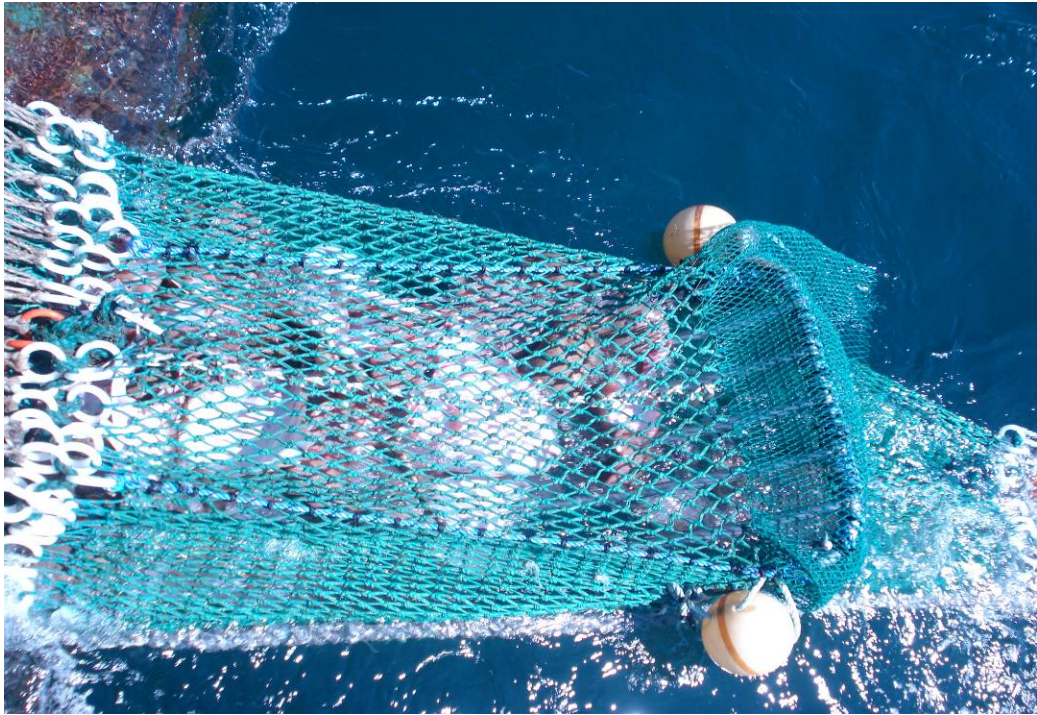
Figure 4a. Photograph of the NMFS flounder TED being hauled back showing the clogging with skates and rays.
