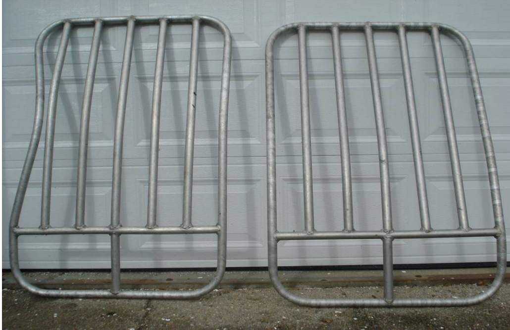
Figure 5a. Photograph of the NMFS certified flounder TED showing the damage from being used.
