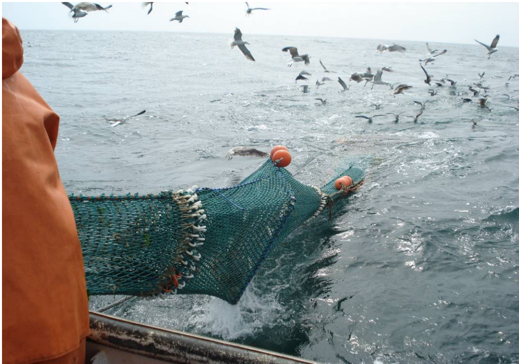
Figure 4b. Photograph of the northeast modified TED during haul-back.
