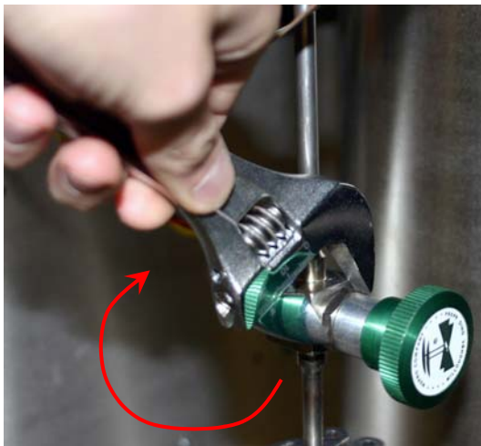
Figure 35 - Loosen Jamb Nut
