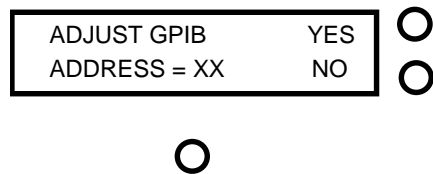
Figure 18 - IEEE-488 Address Adjust Prompt
