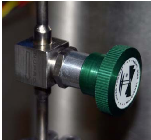
Figure 38 - Tighten Jamb Nut
