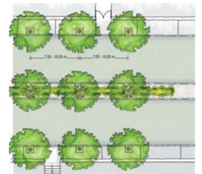
Figure 13: A suggested design for sidewalks and median of a large street.
