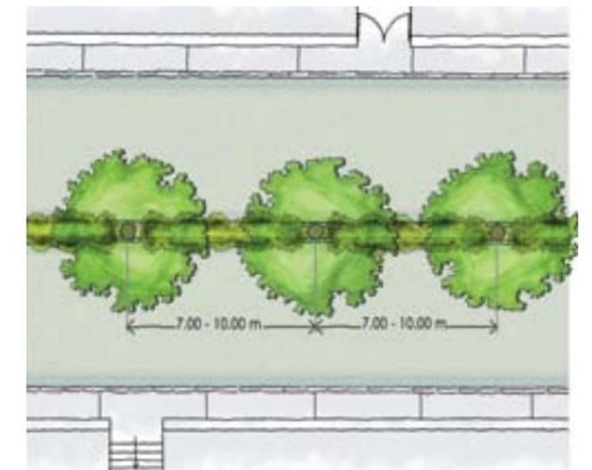
Figure 12: A suggested design for a median of a small street.
