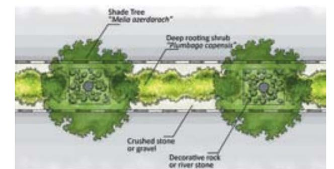
Figure 14: An example of a planting design for a large street median.
