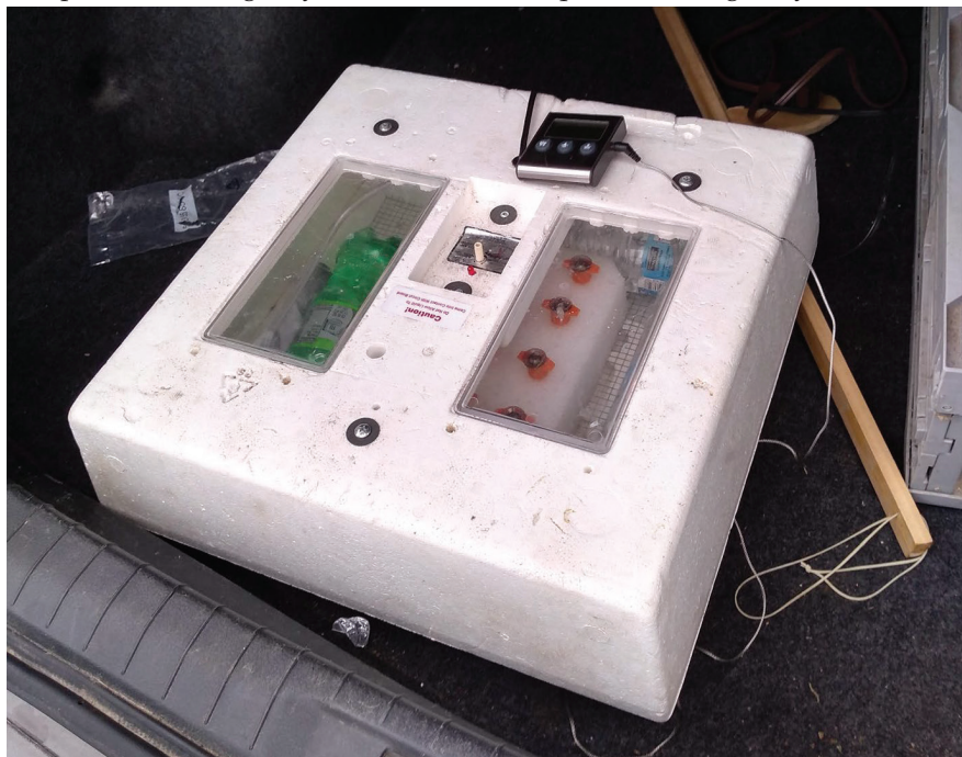
A chicken egg incubator that has been modified to transport queen cells. Incubators work well for long-distance travel. Some are designed to plug right into your vehicle, others can be used with an inverter.
