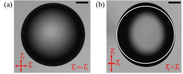
FIG. 4 (color online). (a) Top view of a water droplet atop a SIS film with isotropic tension ( $T_x = T_y$ ). The droplet is round when viewed from above. (b) Top view of a water droplet atop a SIS film which has been stretched in the  $y$  direction ( $T_y > T_x$ ). A white circle is superimposed to emphasize that the droplet is elongated along the direction of high tension. The scale bar represents  $50 \mu\text{m}$ .
