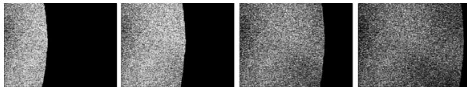
Figure 1. Optical micrographs of a 200-nm PEO film. The time interval between images is 20 s, and each image is 620 \mu\text{m} wide. The sample is crystallized isothermally at 48 ^{\circ}\text{C} .
