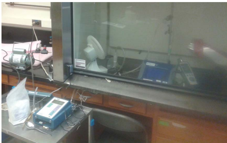
Figure 1. Dust chamber, aerosol generator, and direct reading instruments prior to experiment.
