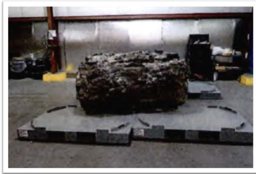
GeoMelt Monolith in Truck Bay (Source: Washington State Department of Ecology, see footnote 57)
