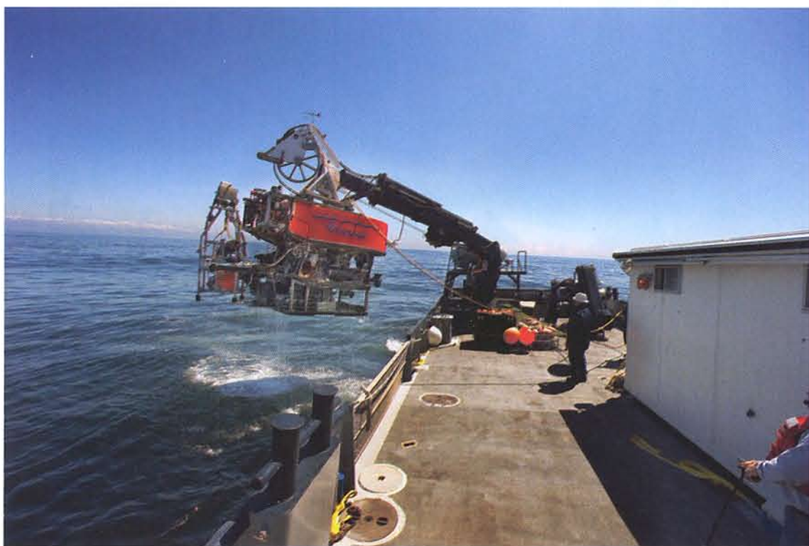
A crane hefts Ventana from Monterey Bay. The submersible clutches the three-legged research device that it retrieved from the seafloor.
