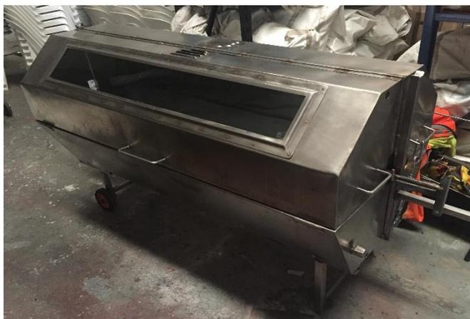
Rotisserie spit: holds up to 55kg, requires LPG & 10amp power outlet. Internal dimensions are 1400mm W x 700mm D x 700mm H. Spit bar cooking length is approx. 1.4m. Includes 5 Prongs.
