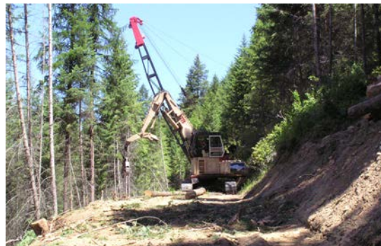
Cable road built appropriately upslope and away from the creek in the Inchelium District.
