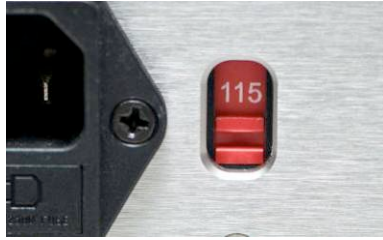
Switch to label "115" for AC100 to 125V voltage.
