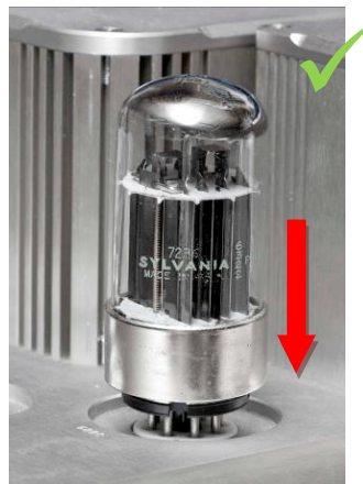
Insert a tube perpendicular to the socket.
