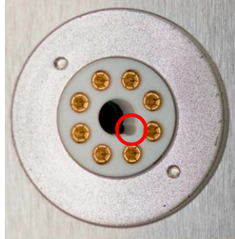
Tube socket guide pin indicator
