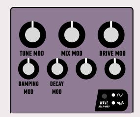
The LFO modulates Tune by default, but you can assign it to other controls. Each knob sets its own modulation amount. At noon, the LFO has no effect. Turn right for positive modulation, and left for negative modulation.
