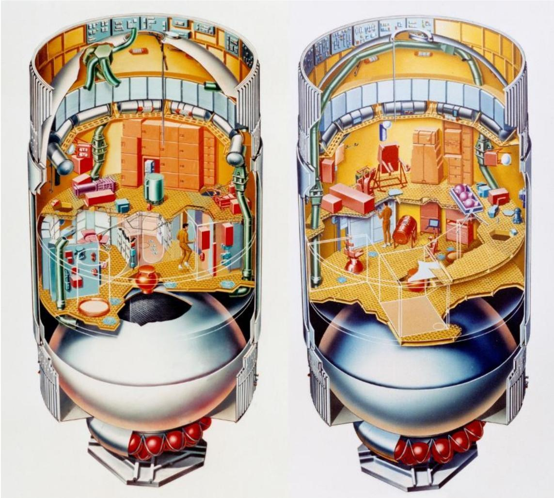
Figure 2. The propellant tanks used to fabricate the Skylab Orbital Workshop are visible in this cutaway schematic of the interior of the station. Photo courtesy of NASA.
