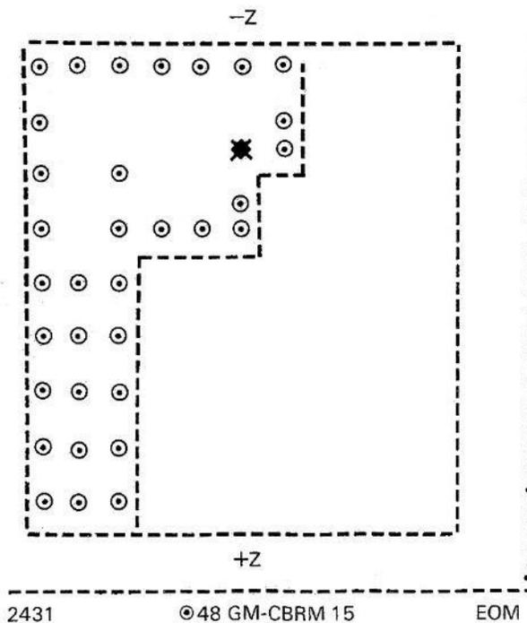
Figure 4. Instructions for the on-orbit repair of a dead power module, radioed to the Skylab 2 crew and accomplished by mission commander Pete Conrad during a spacewalk. Power was restored after he wailed on the battery housing with a hammer. Courtesy of the NASA Historical Reference Collection, Folder 007575; *see also*, Compton and Benson, *Living and Working in Space*.
