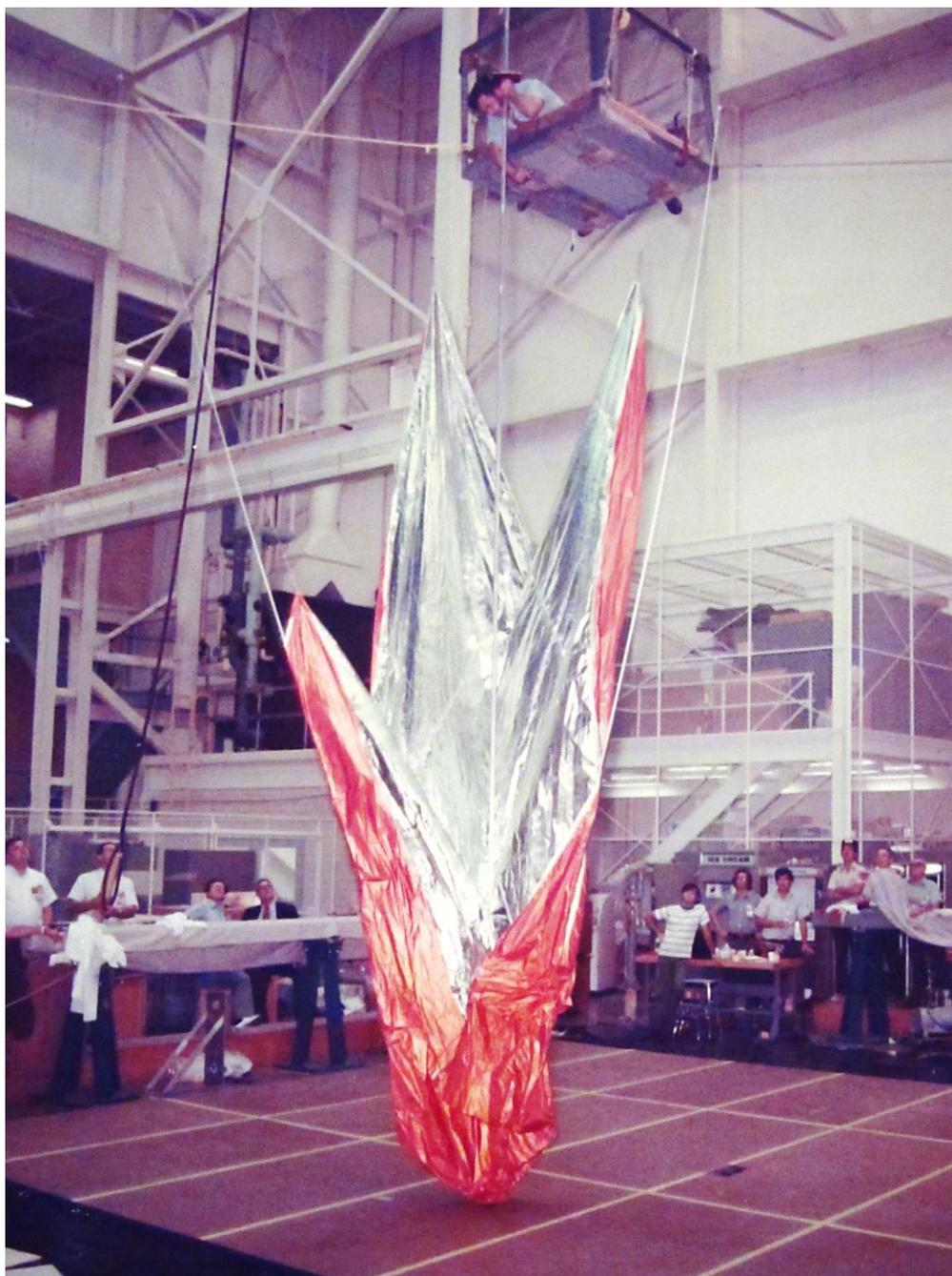
Figure 3. Engineers at NASA's Johnson Space Center test a replacement sunshade for Skylab. Note the ice cream vending machine at rear. Courtesy of the NASA Historical Reference Collection, Folder 007575; see also, W. David Compton and Charles D. Benson, *Living and Working in Space: A History of Skylab* (Washington, D.C.: NASA, 1983).
