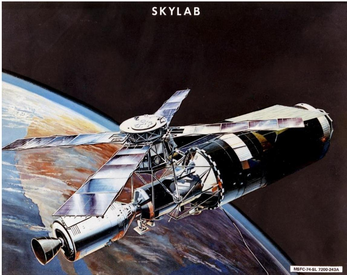
Figure 1. The Skylab Orbital Workshop passes over Baja California in this Marshall Space Flight Center artist's drawing from 1974, depicting the station's actual configuration following the Skylab 3 crew's repairs to the station. Apollo Command and Service Modules are docked at left, and the Apollo Telescope Mount is visible atop the vehicle. At right, the two sun shades installed by the Skylab 2 and 3 crews are visible, one on top of the other. Photo courtesy of NASA.
