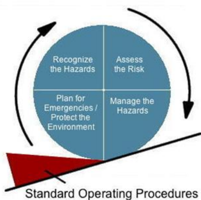
Figure 1: The RAMP paradigm for managing chemical safety in the laboratory. Reprinted by the authors from http://www.irampp.org/blog .
