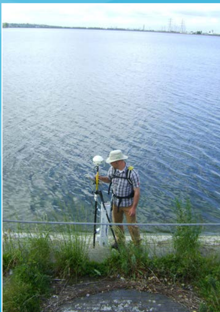
Willowstick reading on the upstream face
