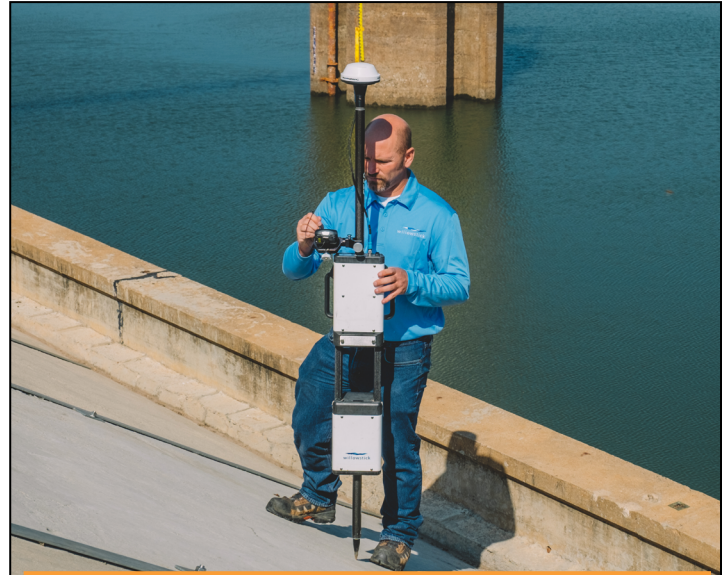
The Willowstick Instrument simultaneously collects magnetic field and GPS Data
