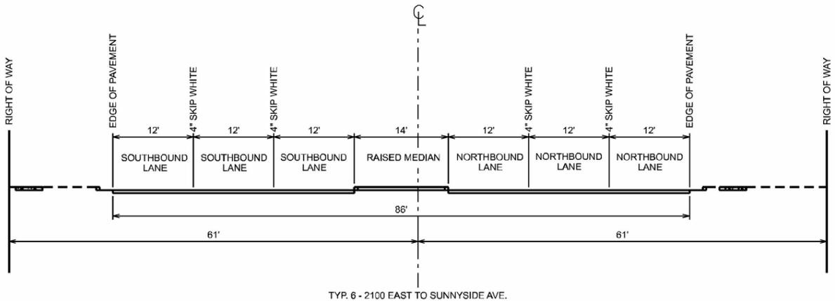
**South of 2100 East** – While there are variations in the cross-section, this segment has a 100 foot right-of-way throughout. From 2100 East to 2300 East, there are six (generally 11-foot) lanes. South of 2300 East, there are four (12-foot) lanes.
