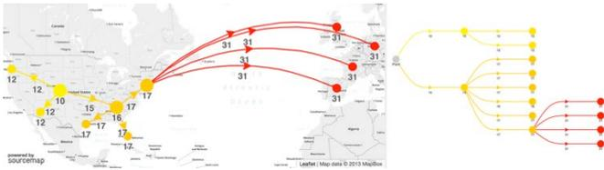
Figure 4. One example of end-to-end supply chain visualization for optimization: landed lead time in days overlaid on a supply chain map (left) and network model (right)
