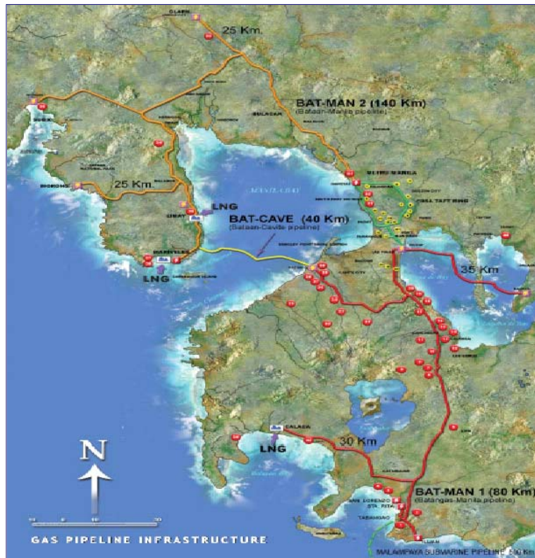
Figure 10-4 Proposed Batangas-Manila Natural Gas Pipeline
