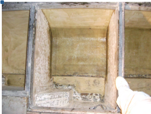
Figure 2: Foam applied and start of fiberglass lay-up to seal Sea King's fish holds
