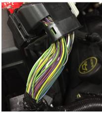
6. Identify the SSB and SSC solenoid wires so that the 6RStager can be inserted into this interface. For 2011-2014 models locate SSB's Green/Brown wire on pin 44 and SSC's Grey/Orange wire on Pin 45 as shown below.
