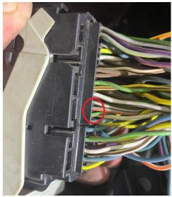
7. Find a good area on the wire harness near the PCM to splice into the SSB signal line coming out of the PCM (Green/Brown) and the SSC signal line coming out of the PCM (Grey/Orange) wire. Connect the wires per the wiring diagrams on pages 2 and 3. Ensure that the wires are connected towards the correct component as shown in the image on the next page.
