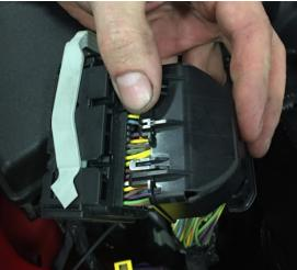
5. Remove at least 6-8 inches of the black tape so that you can access the wires.
