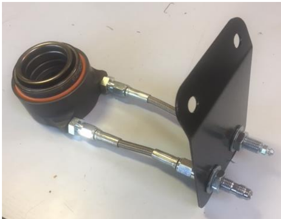
Figure 14 – Throw-out Bearing Sub-Assembly
