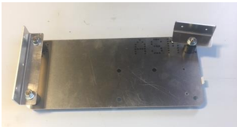
Figure 23 – ECU Mounting Plate Assembly
