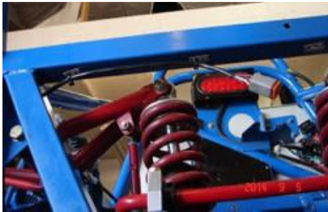
Figure 40 – Tie-wrap tabs for O2 sensor
