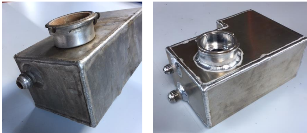
Figure 8 – Un-modified GEN2 & New GEN3 Coolant Tank
