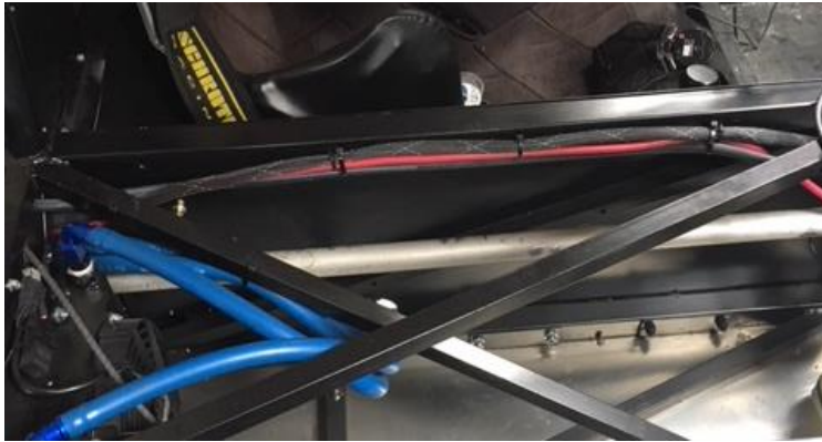
Figure 33 – Tie-Wrap Tab Mounting at Center Section
