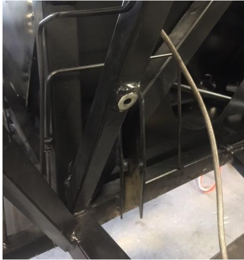
Figure 7 – Transaxle Ground Boss Location
