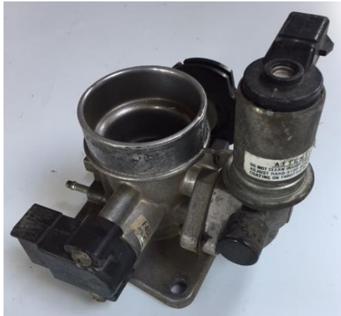
Figure 1 – Throttle Body and IAC
