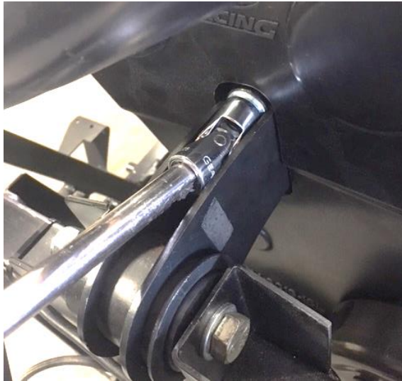
Figure 46 – Tightening the Right Engine Mount Bolts
