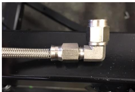
Figure 16 – Modified Clutch Slave Cylinder Hose
