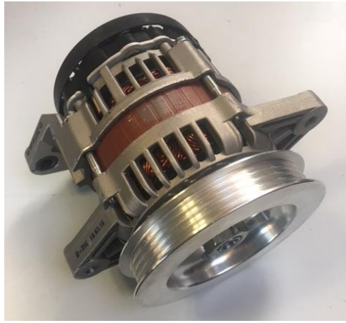
Figure 3 – New Alternator with GEN3 Pulley
