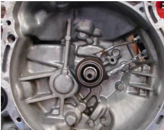
Figure 15 – T/O Bearing & Clutch Lines
