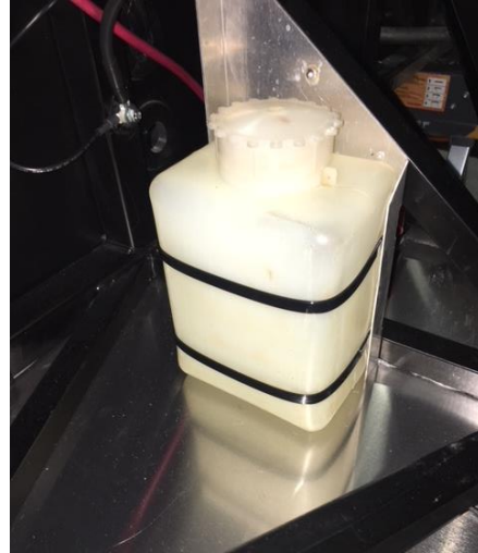
Figure 10 – New Coolant Catch Tank Location
