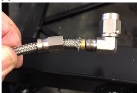
Figure 16 – Modified Clutch Slave Cylinder Hose
